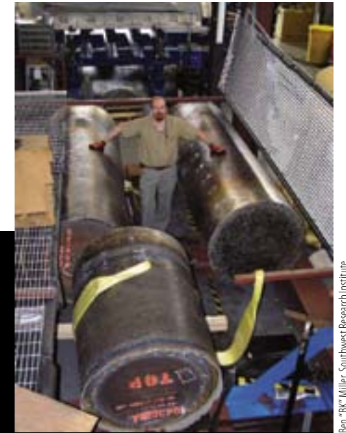
▲ Titanium used to forge the new personnel sphere started out as barrel-shaped ingots fabricated by a mill in Pennsylvania. The two larger ingots, each weighing 17,000 pounds, were shaped into hemispheres that were joined to create the crew compartment. The third ingot, weighing 7,000 pounds, will be used to make viewport and hatch inserts.
